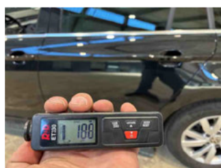
Paint thickness Door RL
