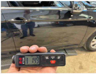
Paint thickness Door FR
