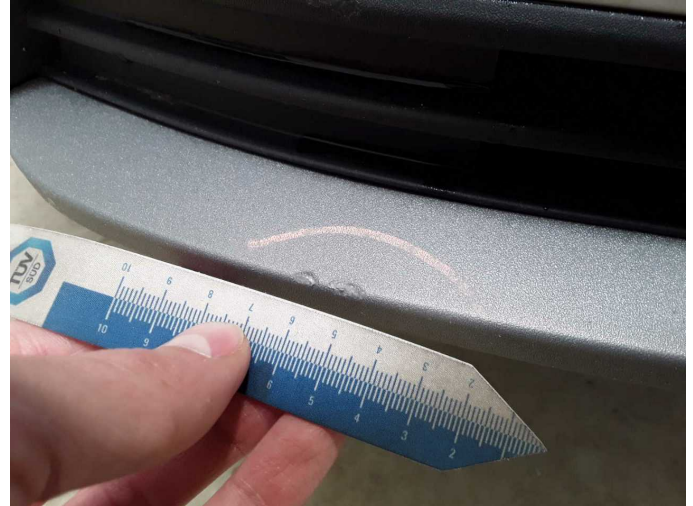
Damage 5: Front bumper: Spoiler - Scratch(es) - Replace
