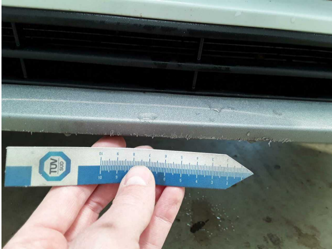
Damage 5: Front bumper: Spoiler - Scratch(es) - Replace
