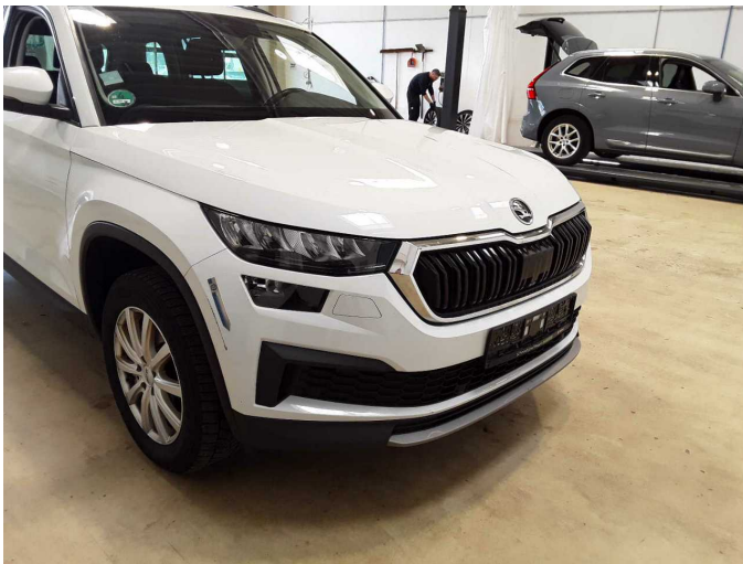
Damage 6: Front bumper: Front bumper - Scratch(es) - Paint
