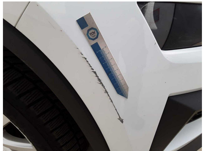
Damage 6: Front bumper: Front bumper - Scratch(es) - Paint
