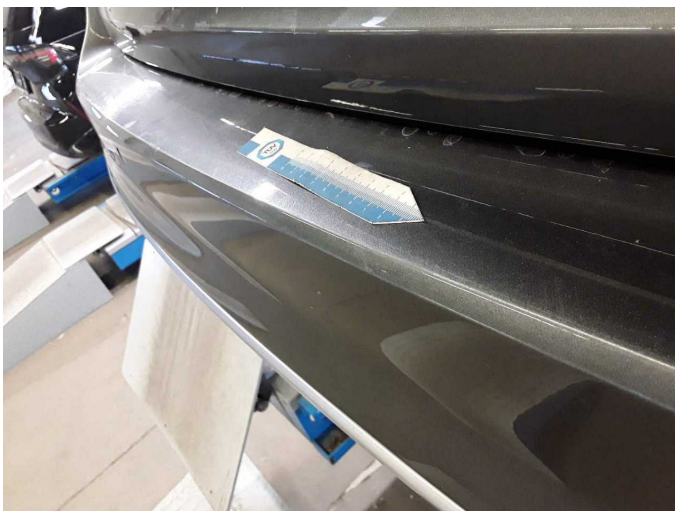
Damage 5: Rear bumper: Rear bumper - Scratch(es) - Paint
