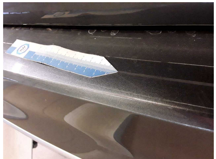
Damage 5: Rear bumper: Rear bumper - Scratch(es) - Paint
