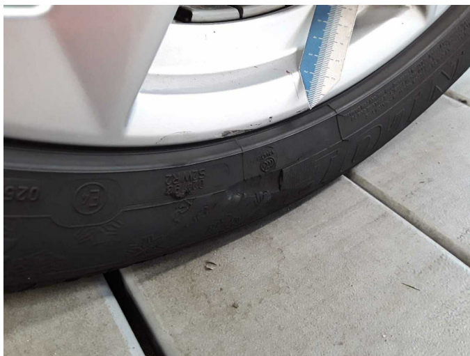
Damage 1: Wheel / tyres: Tyre - front right side - Damaged - Replace
