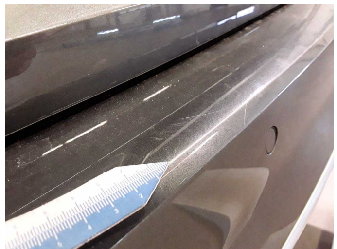
Damage 5: Rear bumper: Rear bumper - Scratch(es) - Paint
