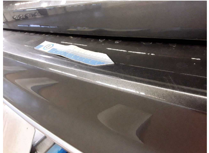
Damage 5: Rear bumper: Rear bumper - Scratch(es) - Paint
