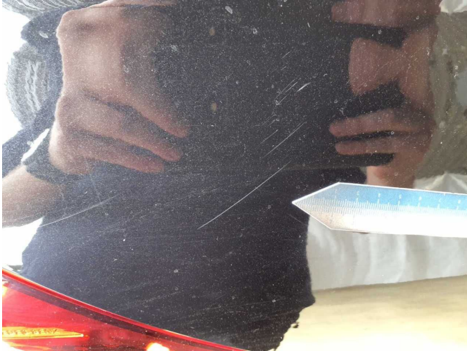
Damage 14: Side panel - rear right side: Side panel - Scratch(es) - Lacquer
