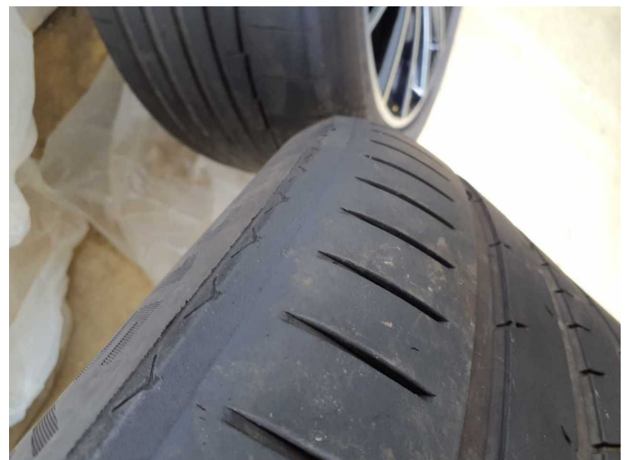
Damage 12: 2nd wheel set: 3 tyres - Does not meet the leasing specifications - Replace
