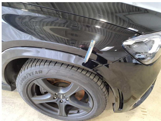
Damage 7: Mudguard - right side: Wheel well extension - Scratch(es) - Paint
