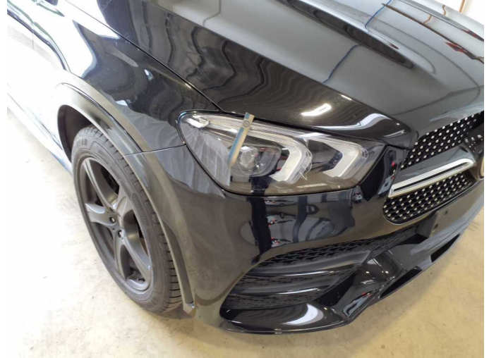
Damage 15: Headlight: Headlight - right side - Scratch(es) - repair according to calculation
