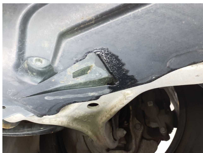
Damage 5: Engine: Engine - Leaking - Perform diagnosis
