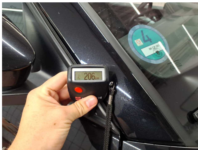
Repainting 1: Roof rail - right side
