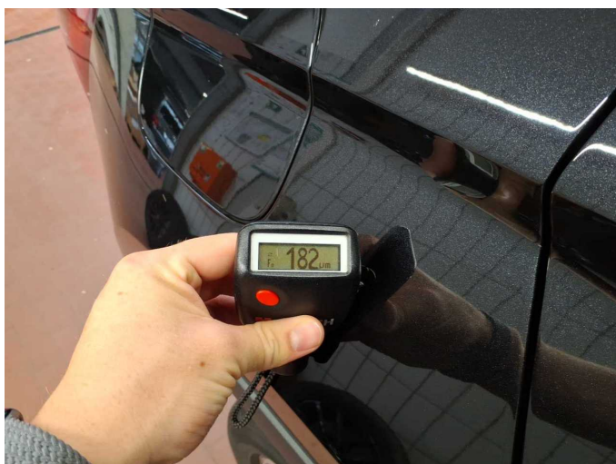
Repainting 2: Side panel - rear right side
