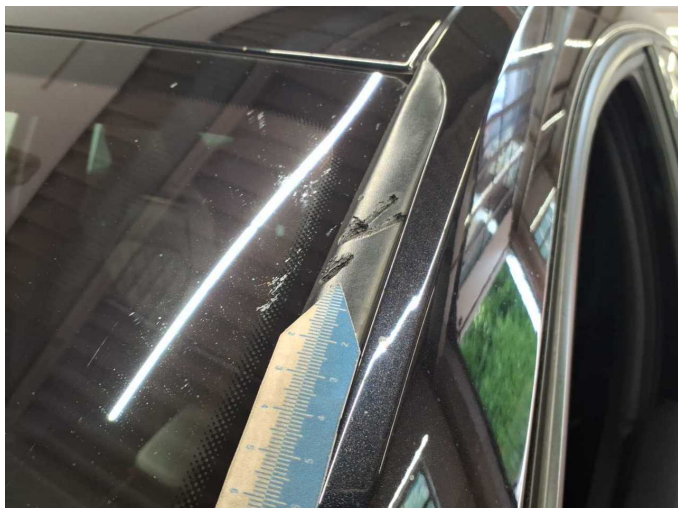
Damage 1: Roof: Cowl - left side - Scratch(es) - Replace
