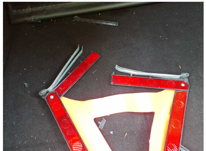
Damage 2: Equipment: Warning triangle - Broken / torn - Replace
