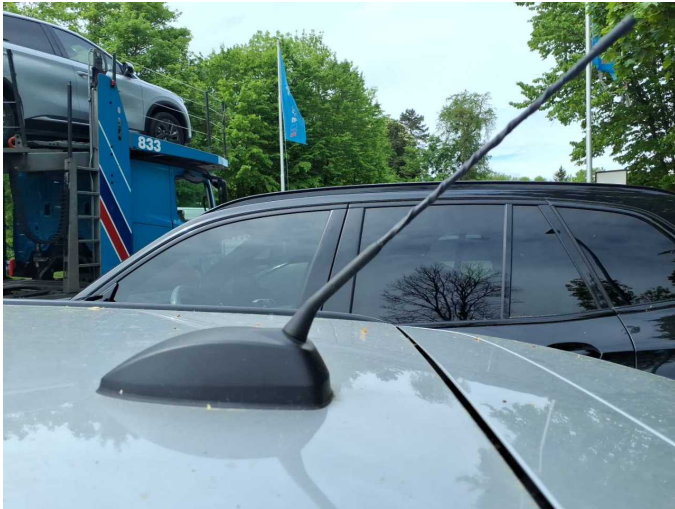
Damage 4: Roof: Stub aerial (Knick) - Broken / torn - Replace
