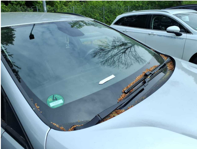
Damage 9: Vehicle glazing: Windscreen - Stone chips - Replace
