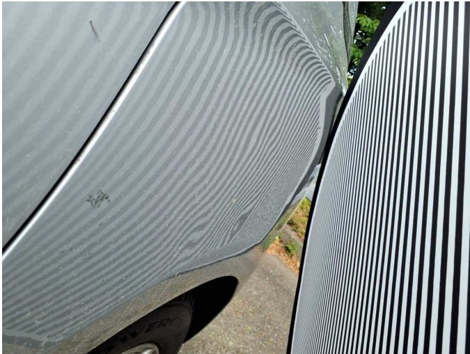
Damage 10: Side panel - rear left side: Side panel - dent(s) - Repair and paint
