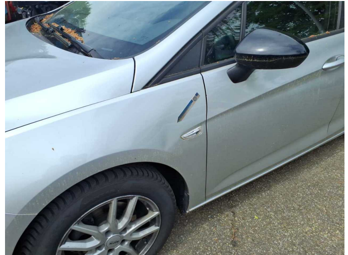
Damage 11: Mudguard - left side: Mudguard - left side - Deformed - Replace
