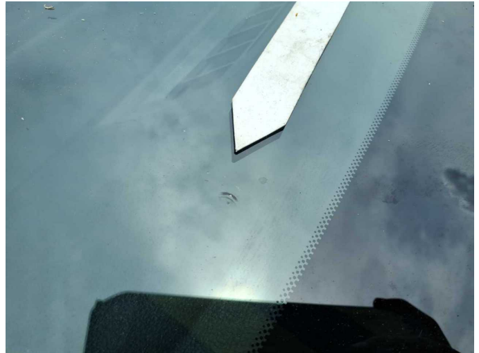
Damage 9: Vehicle glazing: Windscreen - Stone chips - Replace
