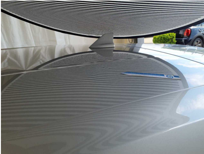
Damage 5: Roof: Roof (Dellen/Wellig) - Deformed - Repair and paint
