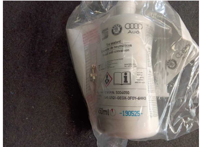
Damage 1: Equipment: Tirefit filler - Expired - Replace
