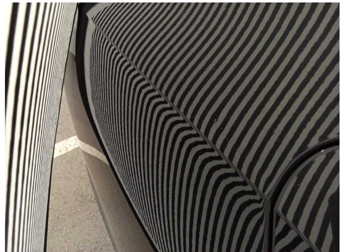
Damage 14: Side panel - rear right side: Side panel - Dent / paintcoat damage - Paint
