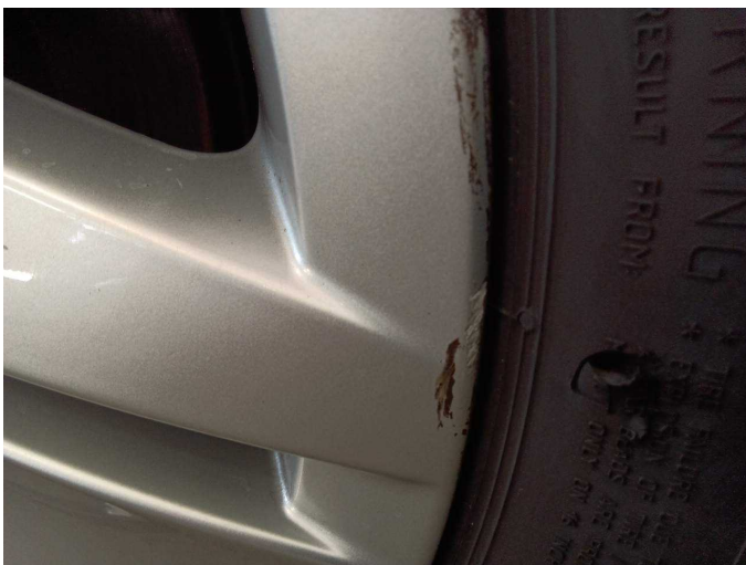
Damage 7: Wheel / tyres: Alloy rim - rear right side - Scratch(es) - Smart repair
