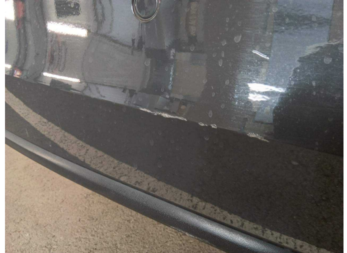
Damage 13: Rear bumper: Rear bumper - Scratch(es) - Paint
