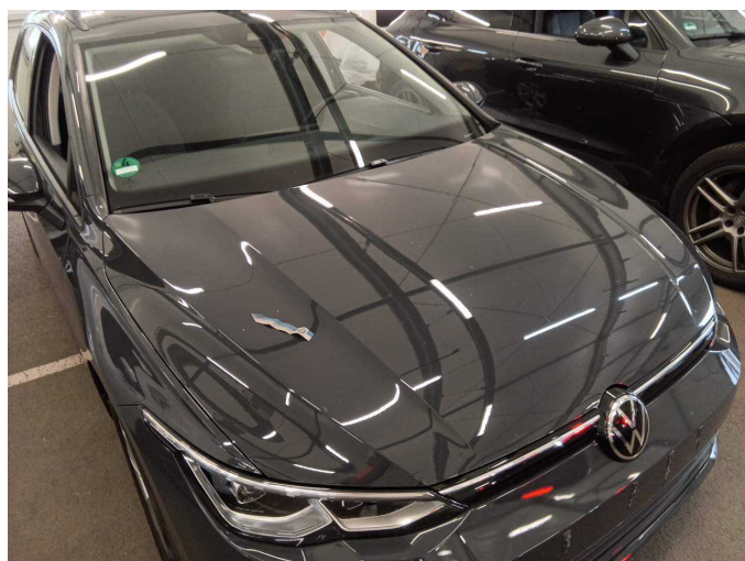
Damage 5: Bonnet: Bonnet - dent(s) - Smooth repair work
