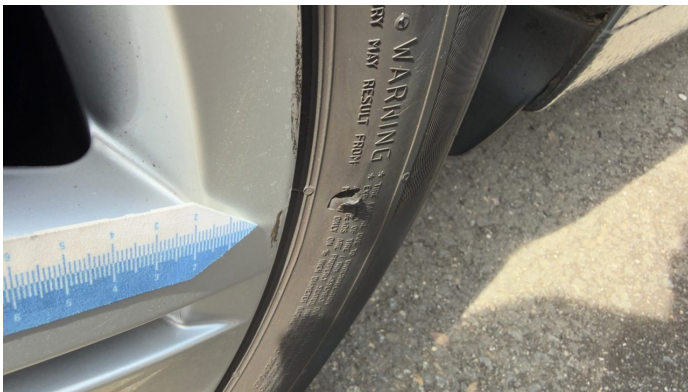
Damage 6: Wheel / tyres: Tyre - rear right side (Flankenbeschädigung) - Damaged - Replace
