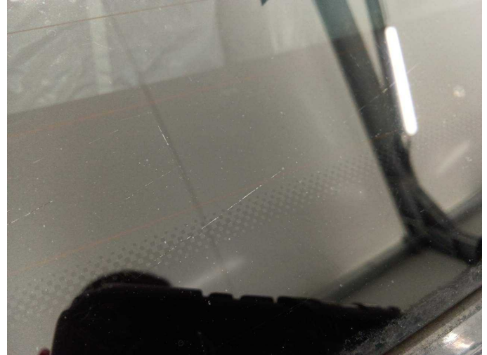
Damage 11: Vehicle glazing: Rear window (Tiefe Kratzer) - Scratch(es) - Replace
