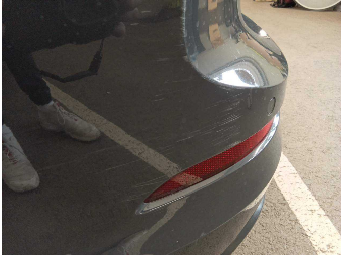
Damage 13: Rear bumper: Rear bumper - Scratch(es) - Paint
