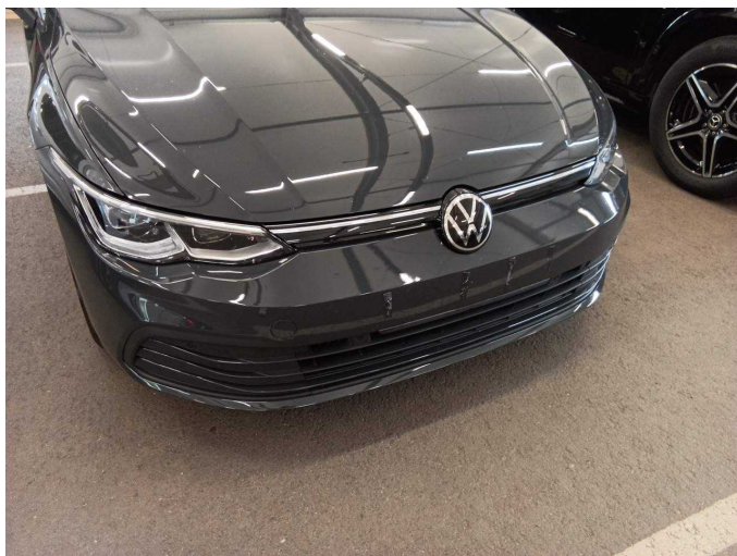
Damage 2: Front bumper: Front bumper (Kleberreste Kennzeichenhalter) - Glued / labelled - De-glue / neutralise
