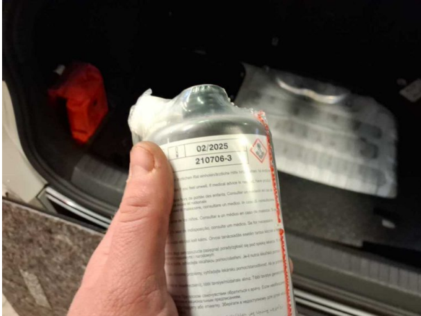
Damage #5: Equipment: Tirefit filler - Expired - Replace
