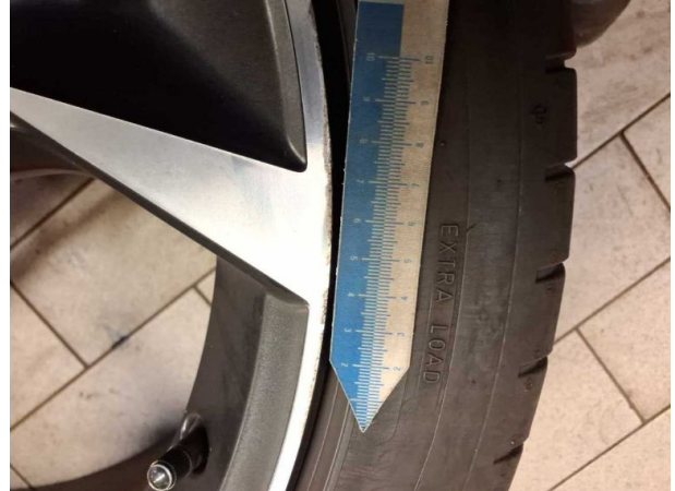
Damage #8: 2nd wheel set: 1 alloy rim - Scratched - Loss in value
