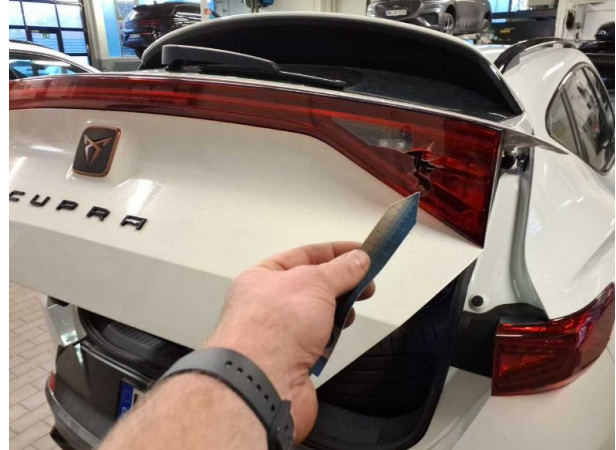
Damage #10: Tail light: Auxiliary brake light - Damaged - Replace
