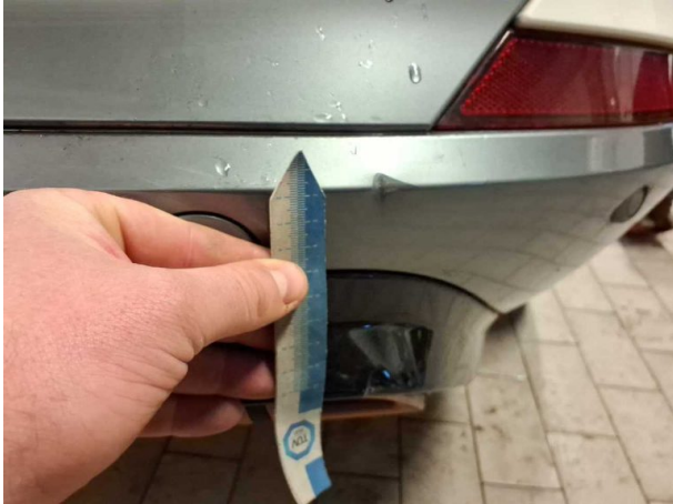
Damage #11: Rear bumper: Rear bumper (Inkl. Spoiler.) - Dent / paintcoat damage - Repair and paint
