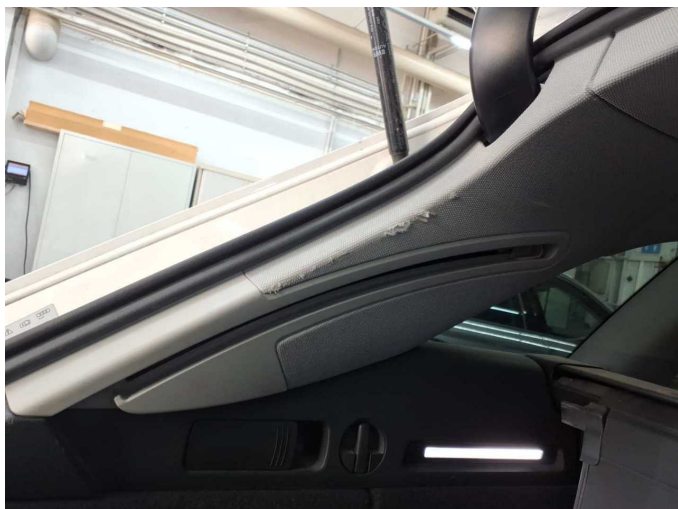
Damage 5: Trim / covers: Boot lining - Holes - Replace
