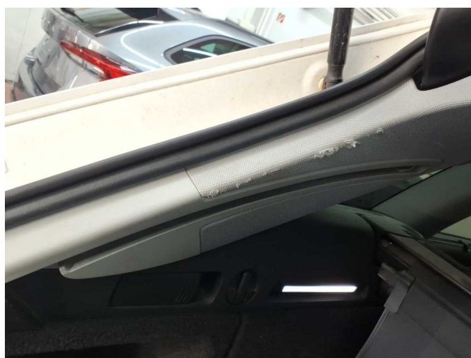
Damage 5: Trim / covers: Boot lining - Holes - Replace
