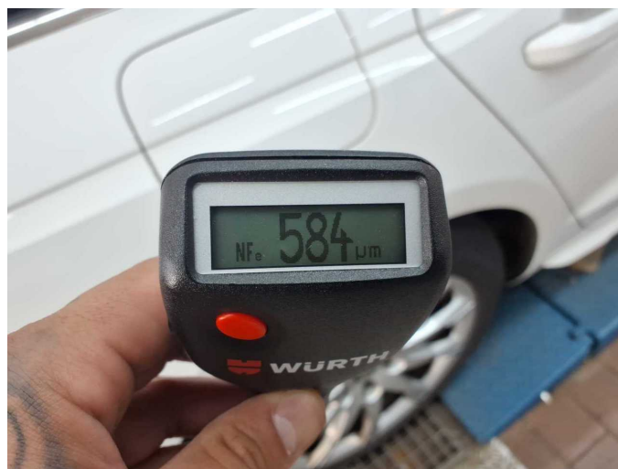
Repainting 1: Side panel - rear right side
