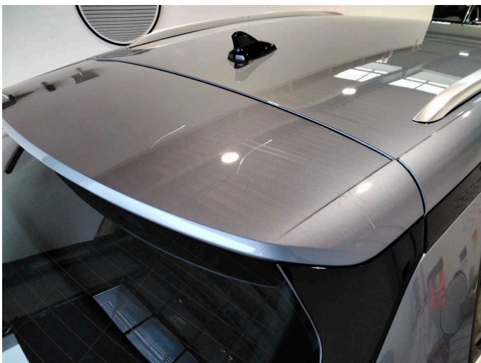
Damage 9: Boot lid / rear door: Boot lid (Spoiler) - Scratch(es) - Paint
