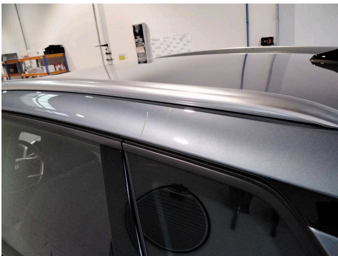
Damage 3: Roof: Roof rail - left side - Scratch(es) - Smart repair
