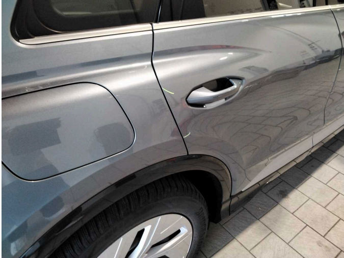
Damage 7: Door - rear right side: Door edge - Scratch(es) - Smart repair
