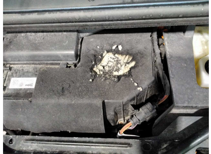
Damage 1: Engine: Engine cover (im vorderen Motorraum) - Damage caused by marten / rodent - Replace
