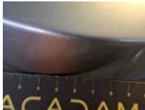
Outside rear-view mirror housing R, Scratch(es), Acceptable
