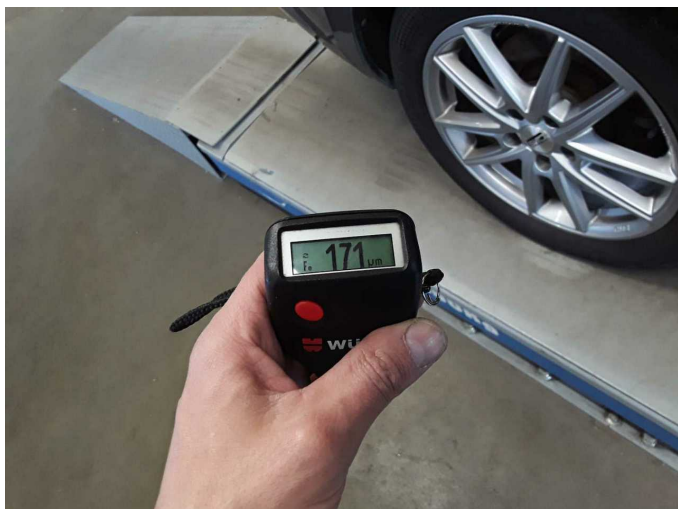
Repainting 1: Side panel - rear right side
