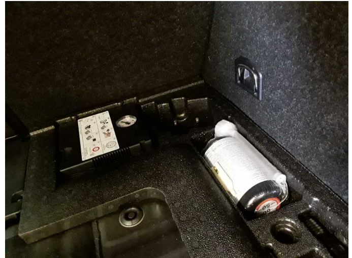
Damage 1: Equipment: Tirefit filler - Expired - Replace
