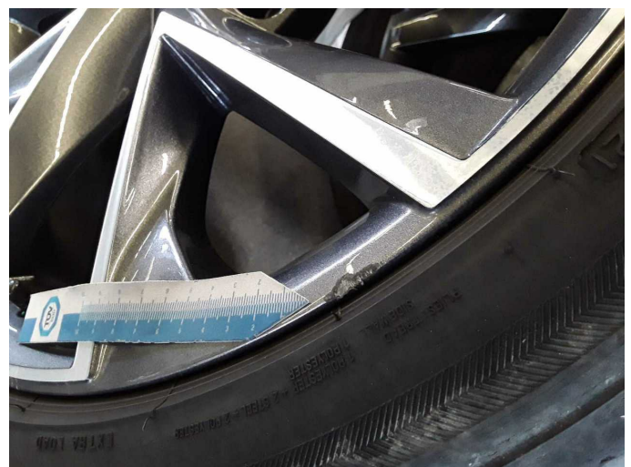
Damage 3: 2nd wheel set: 1 alloy rim - Scratched - Loss in value
