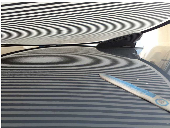
Damage 1: Roof: Roof - dent(s) - Smooth repair work
