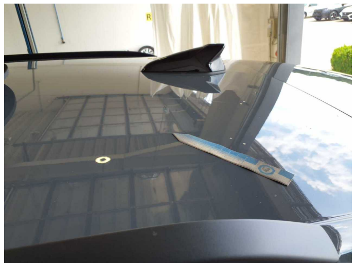
Damage 1: Roof: Roof - dent(s) - Smooth repair work
