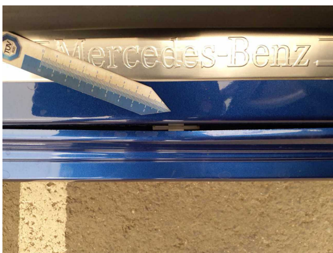
Damage 1: Sill - right side: Trim - Malposition - Un- / install
