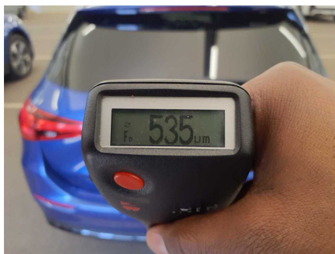
Repainting 1: Boot lid / rear door
