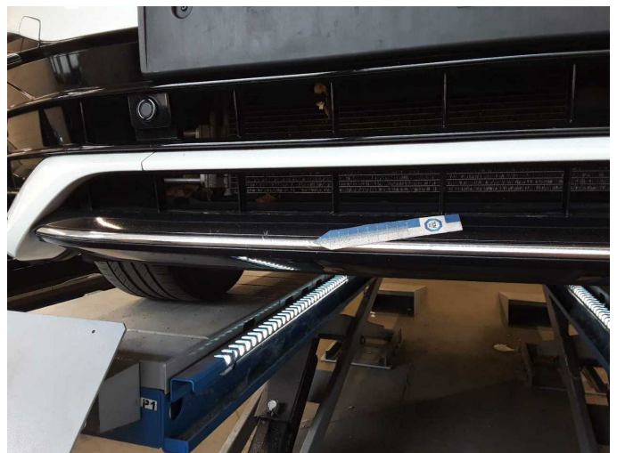
Damage 4: Front bumper: Spoiler (Leiste) - Deformed - Replace
