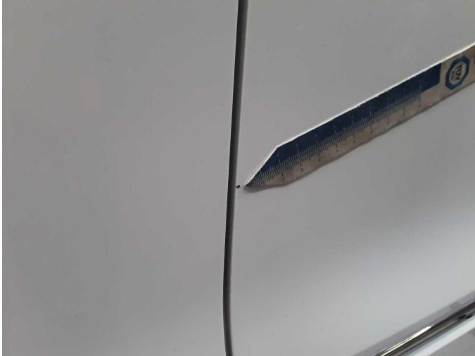
Wear and tear 6: Door - rear left side: Door - Stone chips - No deduction
