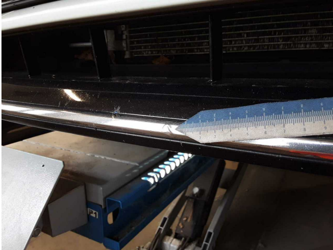
Damage 4: Front bumper: Spoiler (Leiste) - Deformed - Replace
