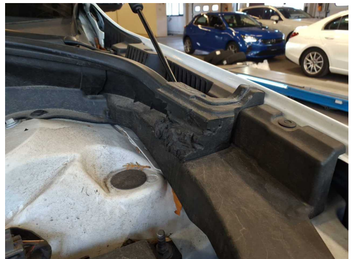
Damage 1: Trim / covers: Trim / covers (Motorraum) - Damage caused by marten / rodent - Replace
