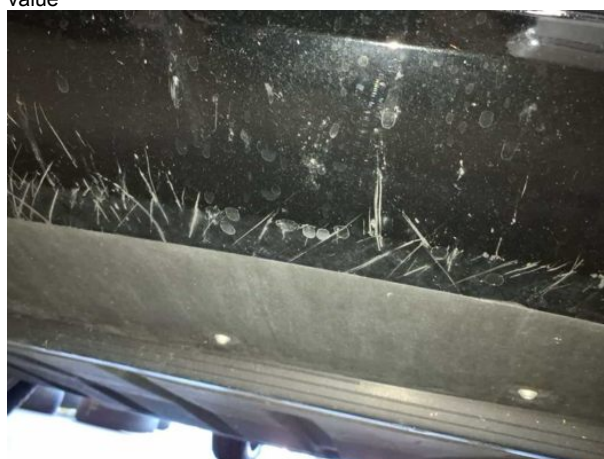
Damage #5: Front bumper: Spoiler - Scratch(es) - Smart repair
