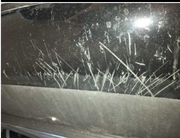
Damage #5: Front bumper: Spoiler - Scratch(es) - Smart repair
