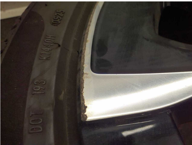
Damage 7: 2nd wheel set: 1 alloy rim - Scratched - Loss in value
