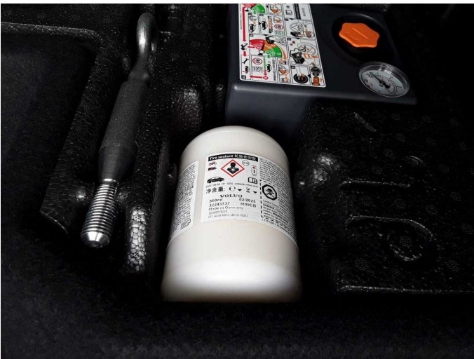
Damage 1: Equipment: Tirefit filler - Expired - Replace
