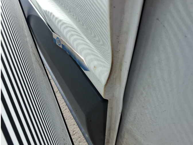
Damage 8: Door - rear right side: Door (Steinschlag mit Korrosion) - Dent / paintcoat damage - Repair and paint
