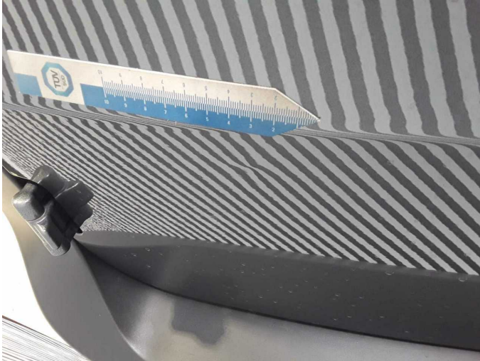
Damage 1: Boot lid / rear door: Rear door - left side - dent(s) - Smart repair
