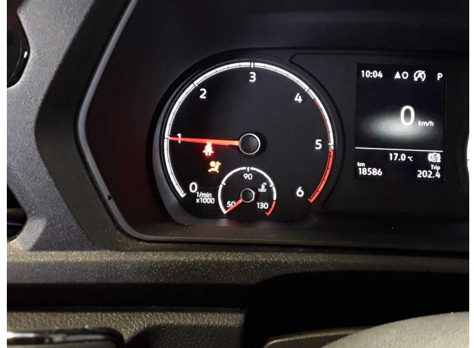
Damage 2: Instrument panel: Indicator light (Airbag) - on - Perform diagnosis
