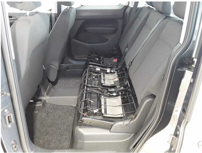
Damage 3: Seat - rear: Seat upholstery - 3 seater bench (inkl. Bezug) - Missing - Replace
