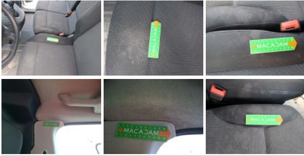
Centre console, Glue residues, Acceptable
