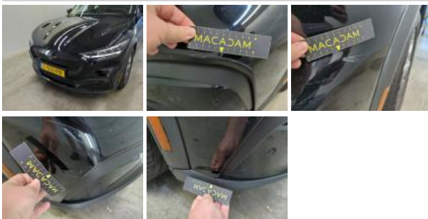
Bumper spoiler F, Scratch(es), Replace
