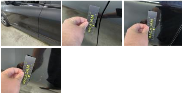
Door RL, Scratch(es), Repair and paint (complete)
