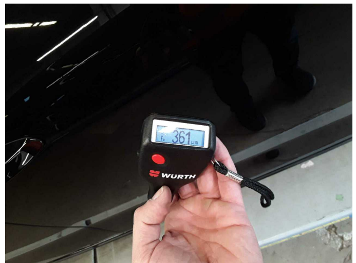
Repainting 1: Roof, Door - front right side
