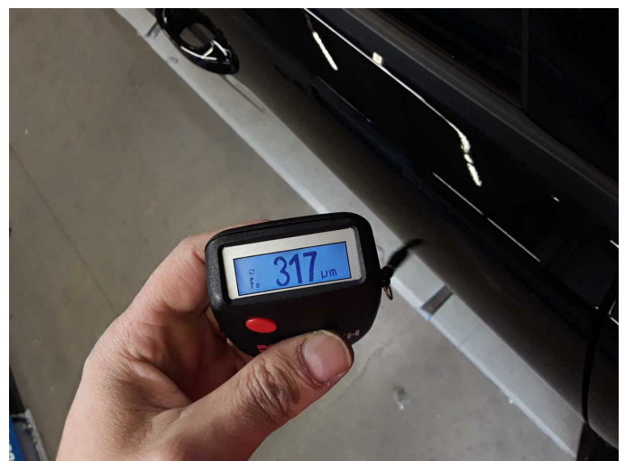
Repainting 1: Roof, Door - front right side
