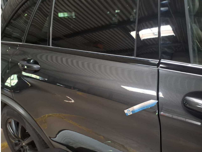
Damage 8: Door - rear right side: Door - Scratch(es) - Smart repair
