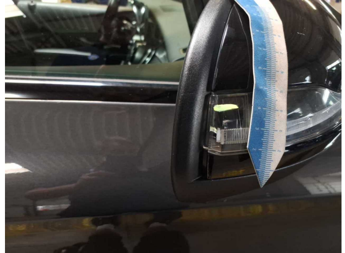
Damage 1: Indicator - front: Mirror - right side - Scratch(es) - Replace
