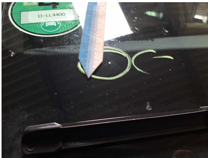
Damage 10: Vehicle glazing: Windscreen - Stone chips - Replace
