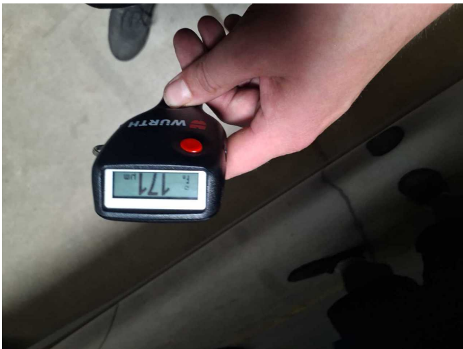
Repainting 1: Door - front left side
