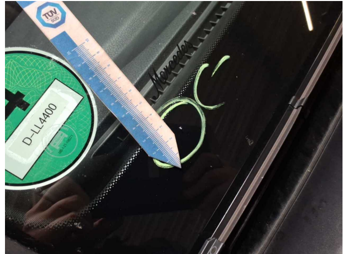
Damage 10: Vehicle glazing: Windscreen - Stone chips - Replace
