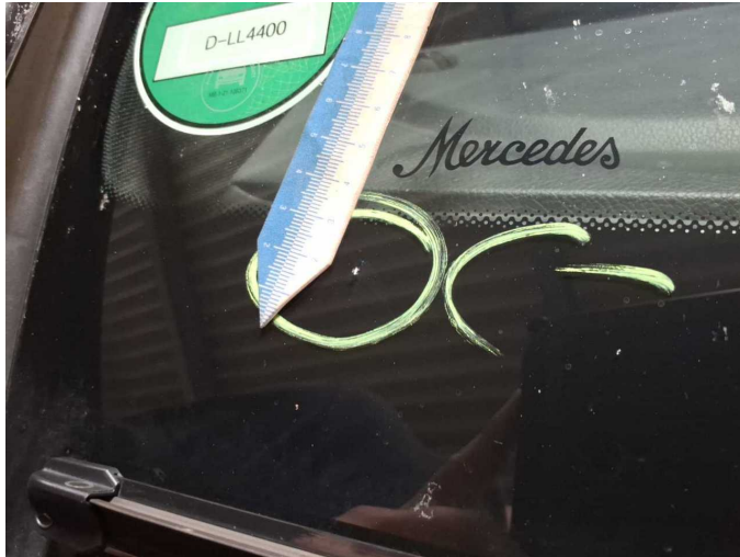
Damage 10: Vehicle glazing: Windscreen - Stone chips - Replace
