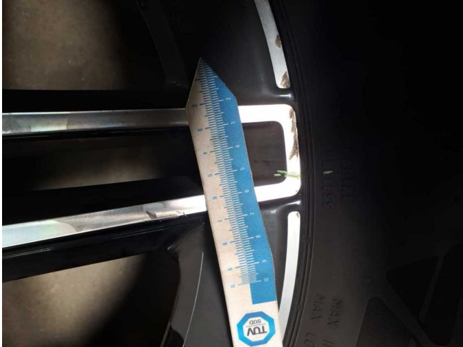
Damage 12: 2nd wheel set: 1 alloy rim - Scratched - Replace
