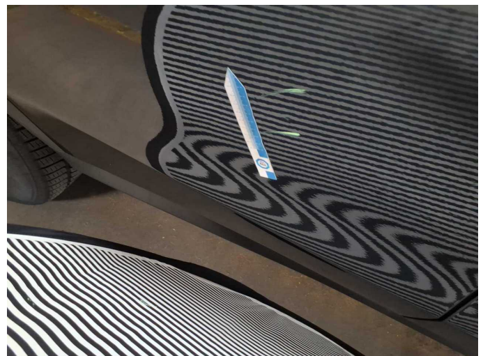
Damage 3: Door - rear right side: Door - Dent / paintcoat damage - Smooth repair work
