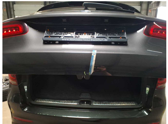
Damage 5: Boot lid / rear door: Boot lid - Scratch(es) - Smart repair
