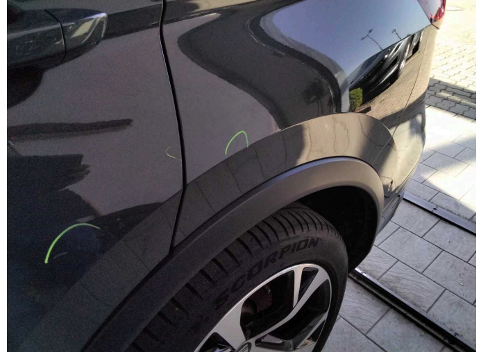
Damage 1: Side panel - rear left side: Side panel - Scratch(es) - Smart repair
