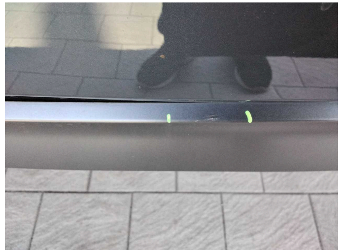
Damage 7: Rear bumper: Spoiler - Scratch(es) - Replace
