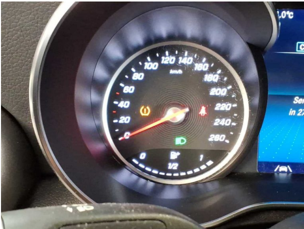
Damage #8: Instrument panel: Indicator light (RDKS brennt) - Specify findings - Perform diagnosis
