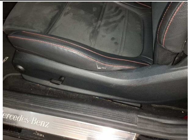
Damage #13: Seat - front: Seat cover - left side - Damaged - Replace
