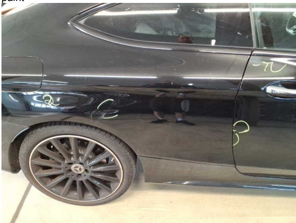
Damage #17: Side panel - rear right side: Side panel - Scratch(es) - Repair and paint
