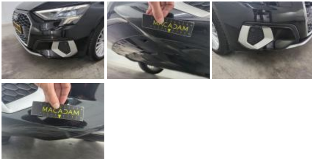
Bumper moulding F, Scratch(es), Replace and paint
