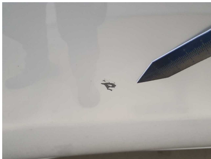
Damage 14: Door - rear right side: Door - Dent / paintcoat damage - Smart repair
