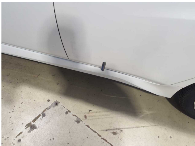
Damage 12: Sill - left side: Trim - Scratch(es) - Smart repair
