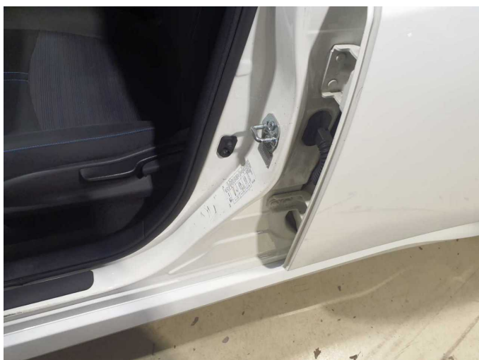
Damage 13: Sill - left side: Sill - Dent / paintcoat damage - Smart repair
