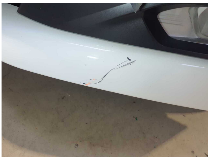
Damage 19: Front bumper: Front bumper - Scratch(es) - Paint
