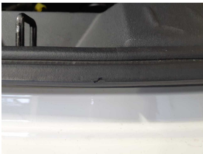
Damage 7: Boot lid / rear door: Seal - Broken / torn - repair/paint (S1)
