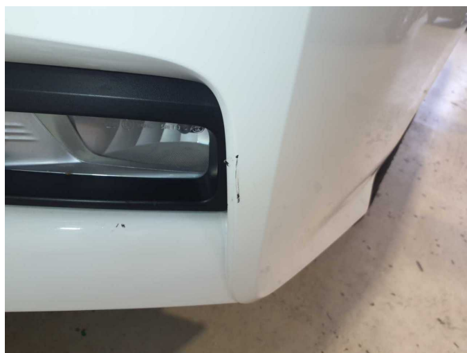
Damage 19: Front bumper: Front bumper - Scratch(es) - Paint
