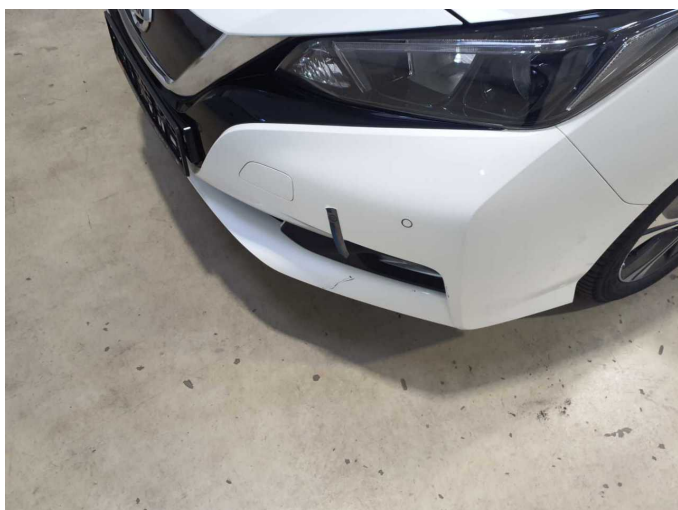
Damage 19: Front bumper: Front bumper - Scratch(es) - Paint
