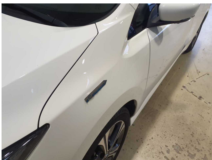
Damage 18: Mudguard - left side: Mudguard - left side (Lack löst sich) - Paint defect - Repair and paint
