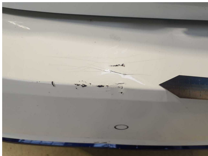
Damage 20: Rear bumper: Rear bumper (Inklusive anbauteile) - Broken / torn - repair according to calculation
