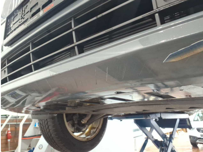
Damage 6: Front bumper: Front bumper - Scratched - Smart repair
