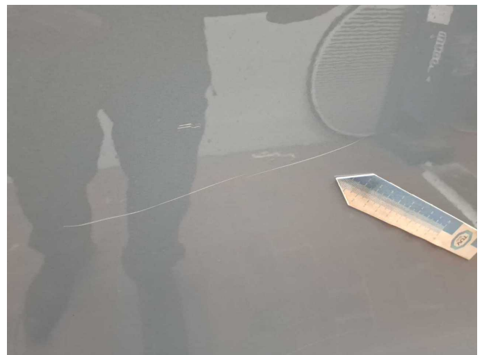
Damage 8: Door - rear right side: Door - Scratch(es) - Repair and paint
