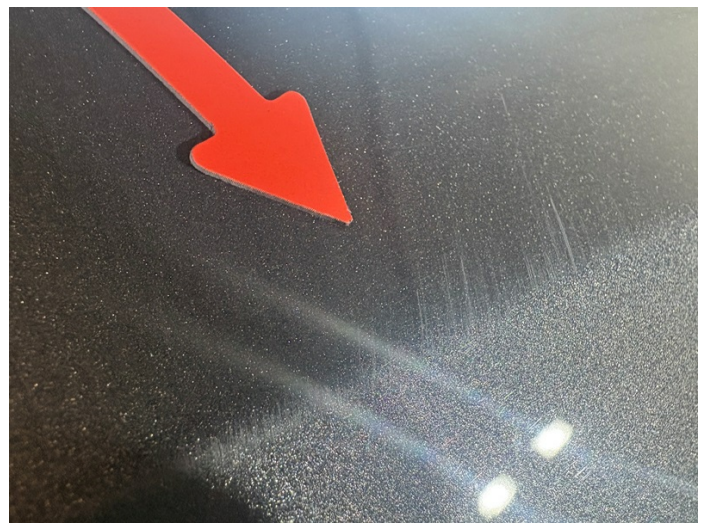
Dachrahmen links: Kratzer (Foto 6)
