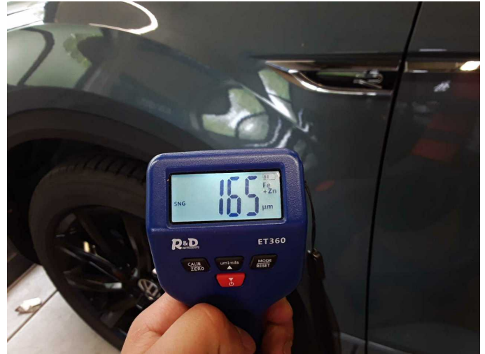
Mudguard - left side: 165 µm
