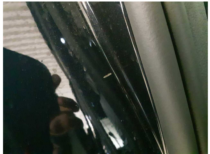
Damage 3: Side panel - rear right side: Sill - Dent / paintcoat damage - Repair and paint
