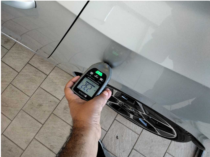
Side panel - rear left side: 232 µm
