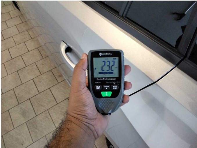
Side panel - rear left side: 232 µm
