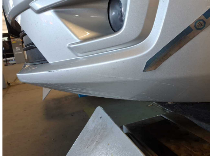
Damage 3: Front bumper: Front bumper - Scratched - Paint
