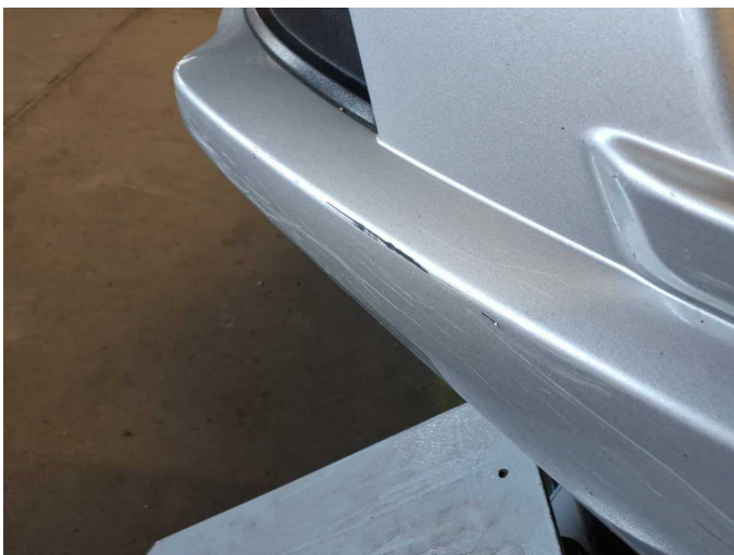
Damage 3: Front bumper: Front bumper - Scratched - Paint
