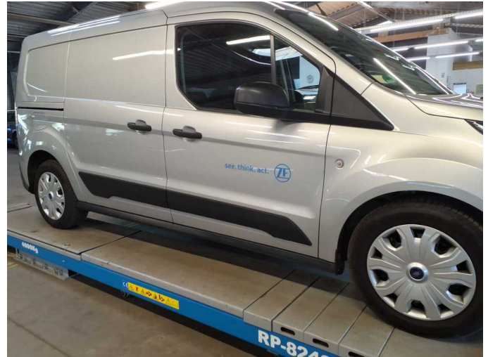
Damage 1: Body: Body - Glued / labelled - De-glue / neutralise
