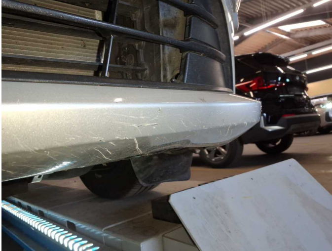
Damage 3: Front bumper: Front bumper - Scratched - Paint
