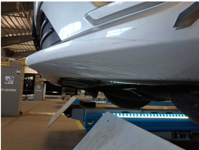
Damage 3: Front bumper: Front bumper - Scratched - Paint
