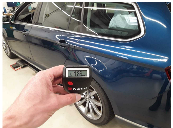
Side panel - rear left side: 1,860 µm
