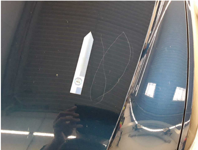
Damage 11: Bonnet: Bonnet - Scratch(es) - Repair and paint
