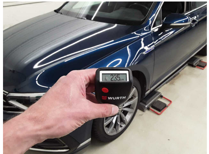
Mudguard - left side: 235 µm
