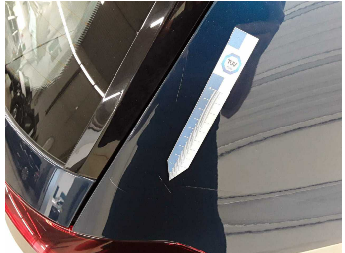
Damage 7: Side panel - rear right side: Side panel - Scratch(es) - Repair and paint
