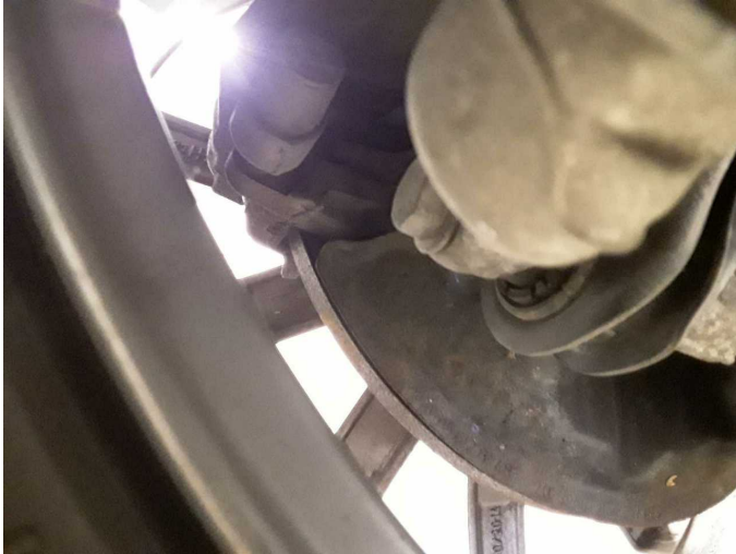
Damage 6: Braking system: Brake discs and pads - rear - Corrosion - Replace
