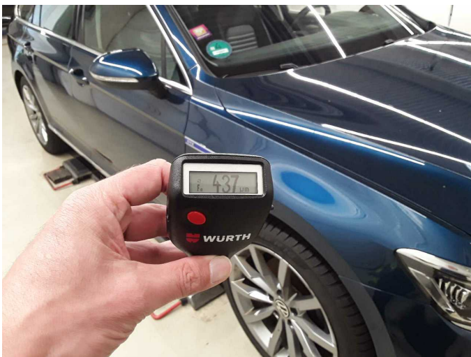
Mudguard - right side: 437 µm
