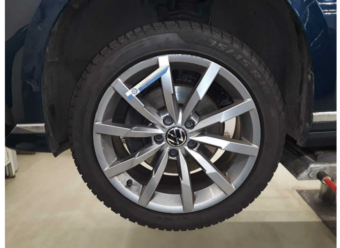
Damage 4: Wheel / tyres: Alloy rim - front left side - Scratched - Loss in value
