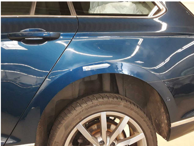
Damage 8: Side panel - rear left side: Side panel - Scratch(es) - Repair and paint
