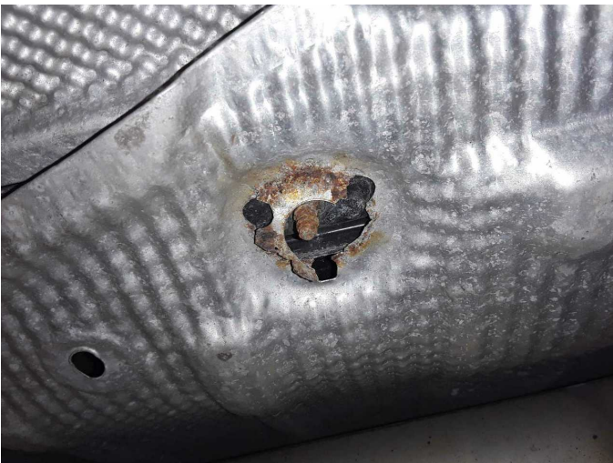
Damage 2: Exhaust system: Heat shield (Lose , hinten ,mitte) - Broken / torn - Replace
