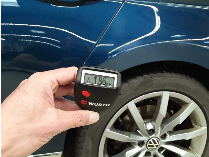
Side panel - rear left side: 1,860 µm
