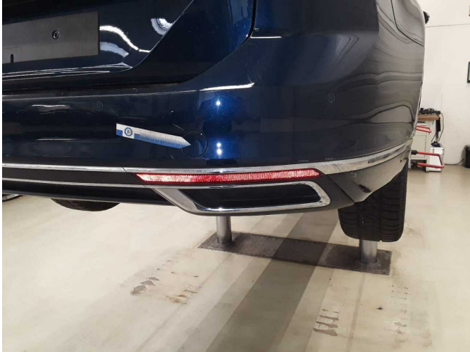
Damage 12: Rear bumper: Rear bumper (Incl. Anbauteile, Chrom erneuern,) - Scratched - Repair and paint
