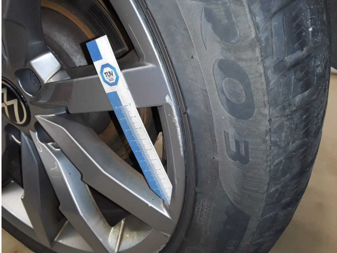
Damage 3: Wheel / tyres: Alloy rim - rear left side - Scratched - Loss in value
