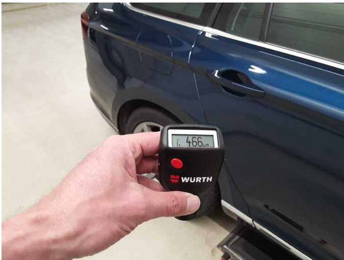
Side panel - rear right side: 466 µm
