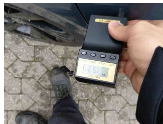
Paint thickness Door RR
