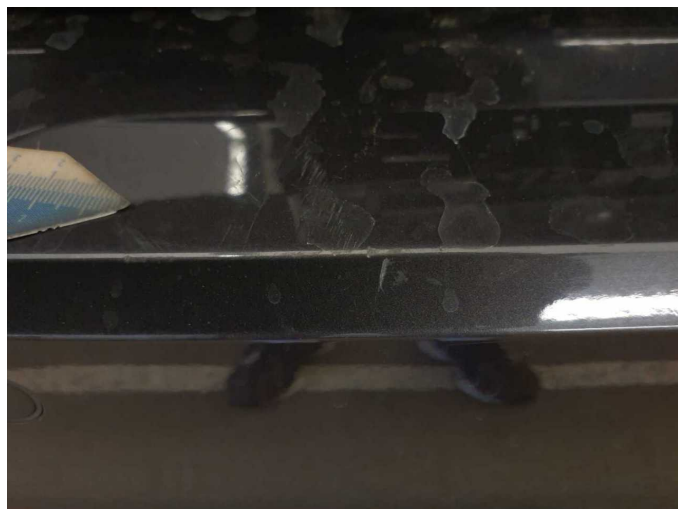
Damage 5: Rear bumper: Rear bumper - Scratch(es) - Paint
