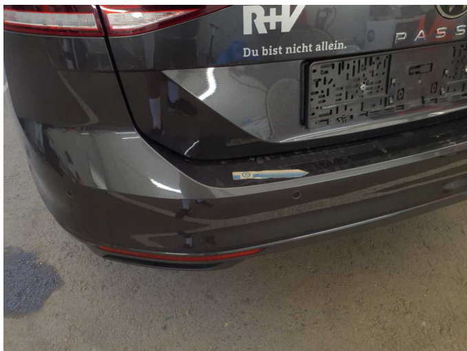
Damage 5: Rear bumper: Rear bumper - Scratch(es) - Paint
