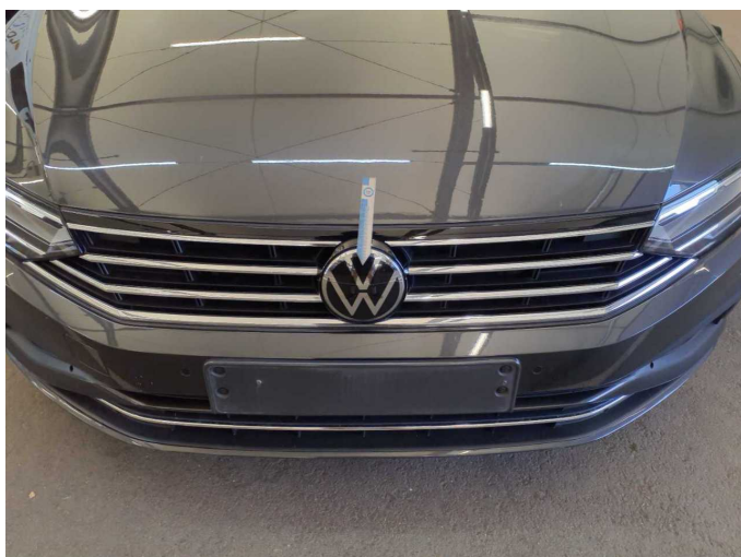
Damage 4: Front structure: Emblem - Broken / torn - Replace
