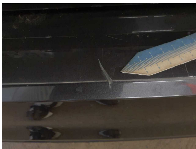
Damage 5: Rear bumper: Rear bumper - Scratch(es) - Paint
