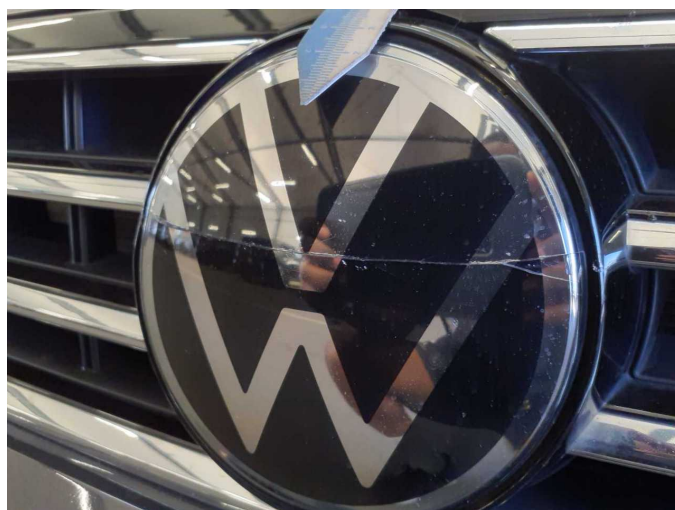
Damage 4: Front structure: Emblem - Broken / torn - Replace
