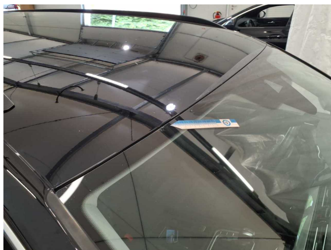
Damage 7: Vehicle glazing: Windscreen (kein Staubschutz) - Broken / torn - repair according to calculation
