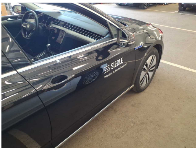
Damage 2: Body: Body - Glued / labelled - De-glue / neutralise
