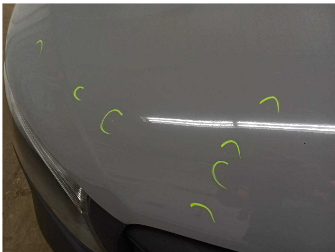
Damage 5: Bonnet: Bonnet - Stone chips - Paint
