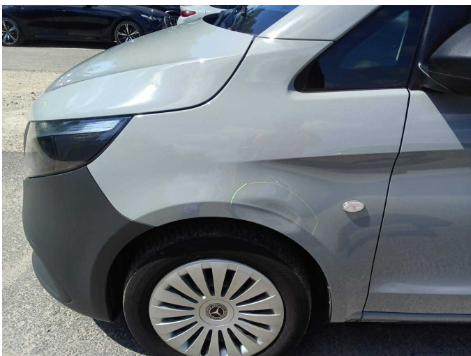
Damage 3: Mudguard - left side: Mudguard - left side - Dent / paintcoat damage - Repair and paint
