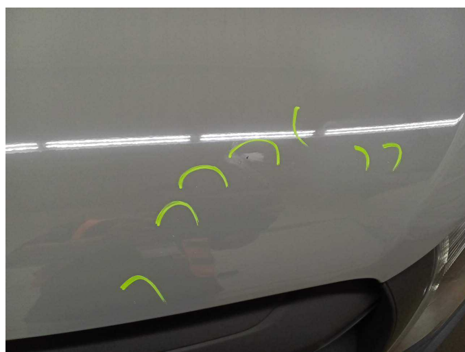
Damage 5: Bonnet: Bonnet - Stone chips - Paint
