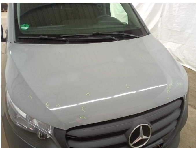
Damage 5: Bonnet: Bonnet - Stone chips - Paint
