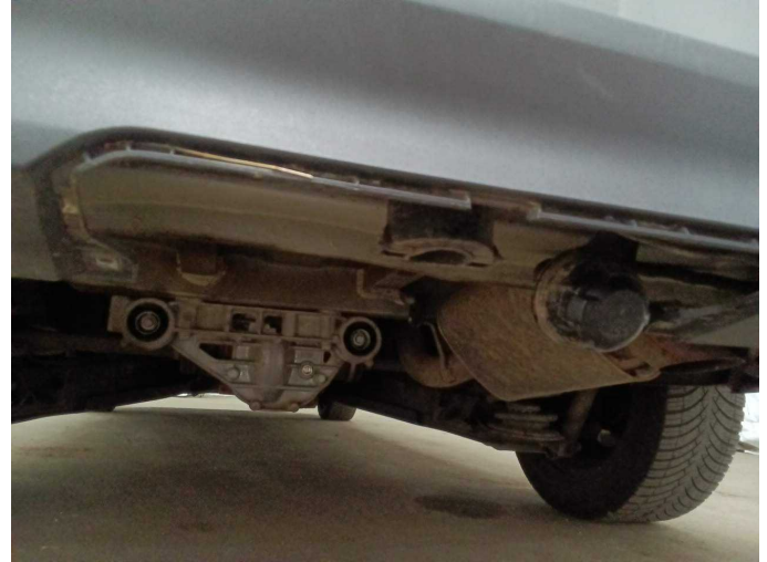
Damage 1: Trim / covers: Trim / covers - Missing - Replace
