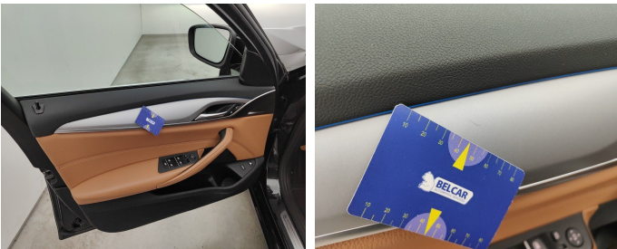
Front Left Door Interior Coating // Replace Completely-scratch
