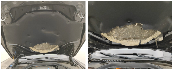
Front Bonnet / Insulation / Replace-tear
