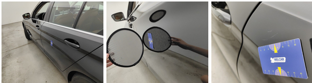
Door Rear Left // Smart Repair Small-dent
