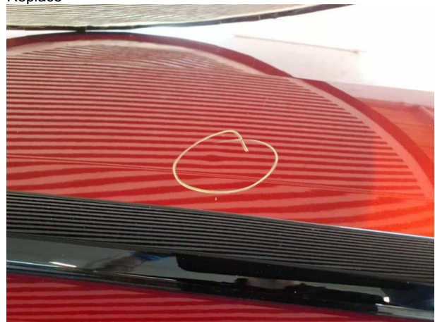
Damage #11: Roof: Roof - dent(s) - Smooth repair work
