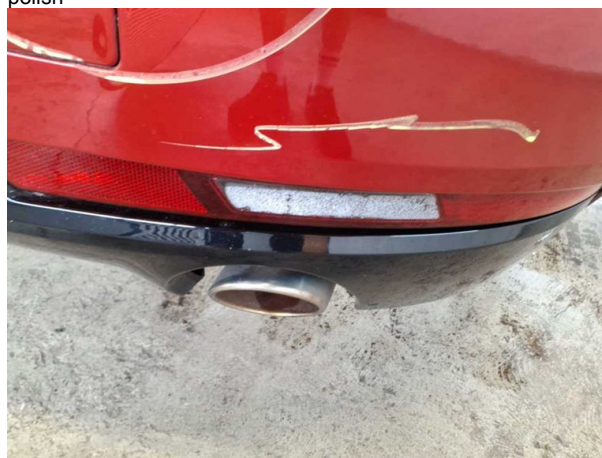
Damage #4: Boot lid / rear door: Reflectors - Leaking - Replace
