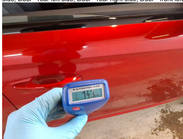
Repainting 1: Side panel - rear left side, Side panel - rear right side, Door - rear left side, Door - rear right side, Door - front left
