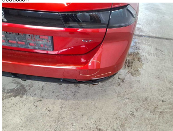
Damage #2: Rear bumper: Rear bumper - Scratched - Cover / polish
