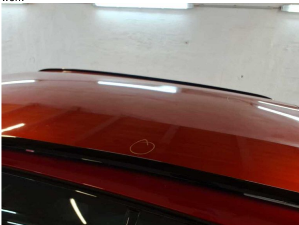
Damage #11: Roof: Roof - dent(s) - Smooth repair work
