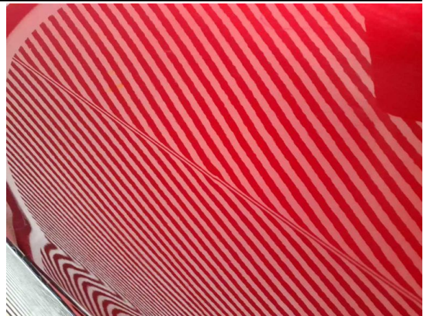
Damage #9: Door - rear right side: Door - dent(s) - Smooth repair work
