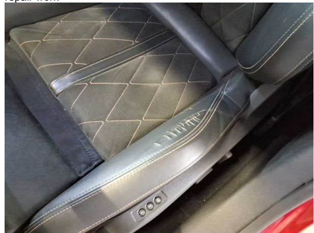
Damage #10: Seat - front: Seat cover - left side - Damaged - Replace
