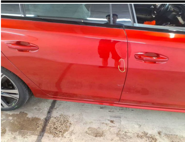
Damage #9: Door - rear right side: Door - dent(s) - Smooth repair work
