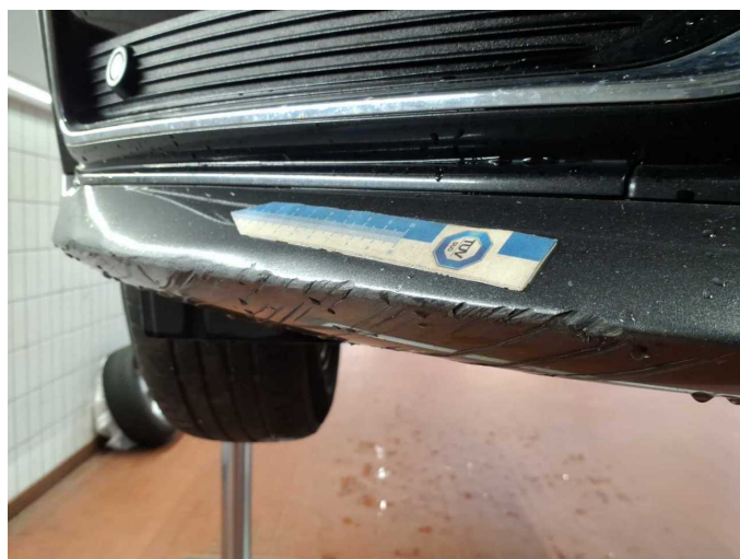
Damage 7: Front bumper: Spoiler - Scratched - Paint
