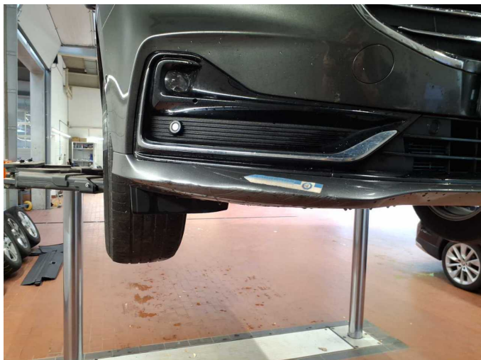
Damage 7: Front bumper: Spoiler - Scratched - Paint
