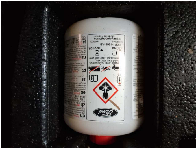
Damage 1: Equipment: Tirefit filler - Due - Replace
