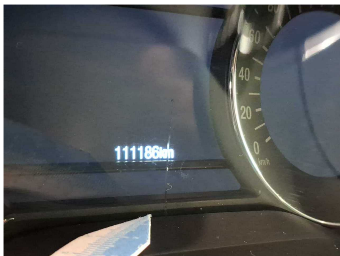
Damage 9: Instrument panel: Instrument cluster (Scheibe) - Broken / torn - repair according to calculation
