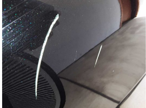
Damage #1: Door - rear left side: Door - Scratch(es) - Cover / polish
