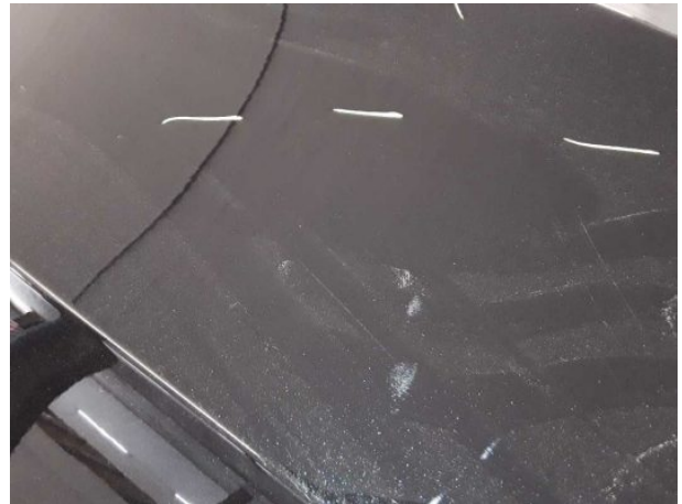
Damage #12: Bonnet: Bonnet - Scratched - Repair and paint
