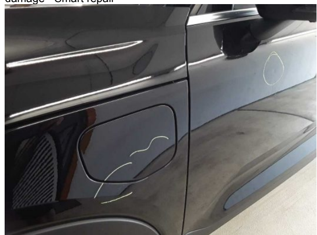
Damage #5: Fuel system: Tank cap - Scratched - Smart repair
