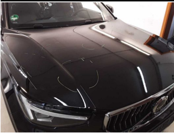
Damage #12: Bonnet: Bonnet - Scratched - Repair and paint
