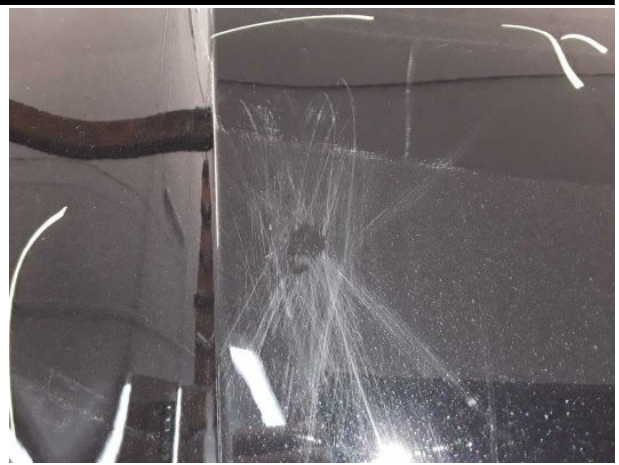
Damage #12: Bonnet: Bonnet - Scratched - Repair and paint
