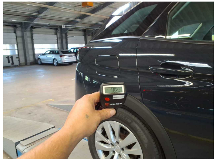
Repainting 6: Side panel - rear right side
