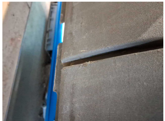
Damage 4: Door - front right side: Brightware - lower - Scratch(es) - Smart repair
