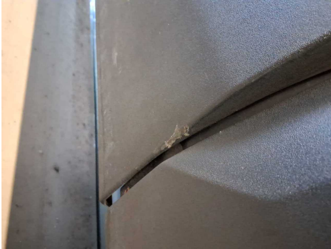
Damage 5: Door - front left side: Brightware - lower - Scratch(es) - Smart repair
