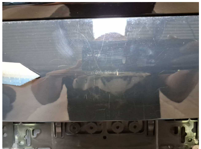
Damage 10: Boot lid / rear door: Boot lid - Scratched - Repair and paint
