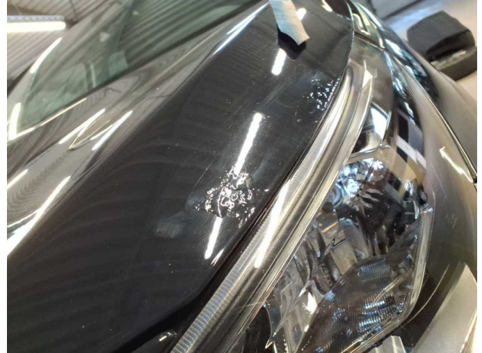
Damage 9: Bonnet: Bonnet - Corrosion - Repair and paint
