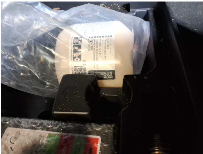
Damage 1: Equipment: Tirefit filler - Expired - Replace
