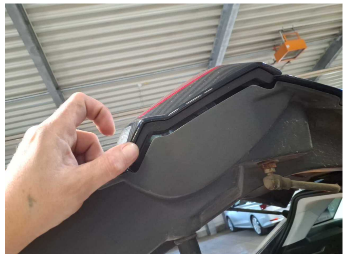
Damage 2: Tail light: Tail lamp - right side (Heckklappe, evtl. erneuern) - Loose - Un- / install
