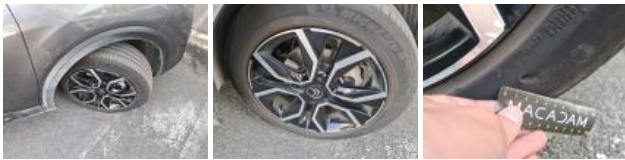
Tyre FL, Tear, Replace
