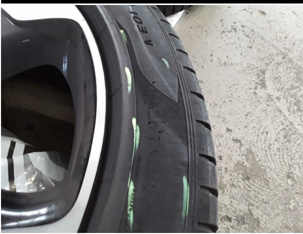
Damage #8: Wheel / tyres: Tyre - front - Damaged - Replace
