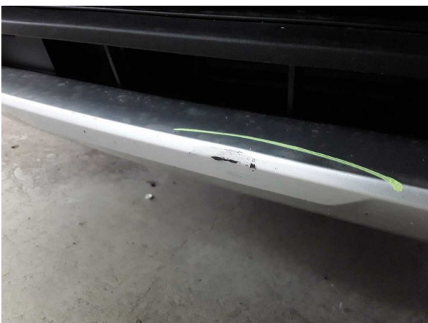
Damage #7: Front bumper: Spoiler - Scratched - Smart repair
