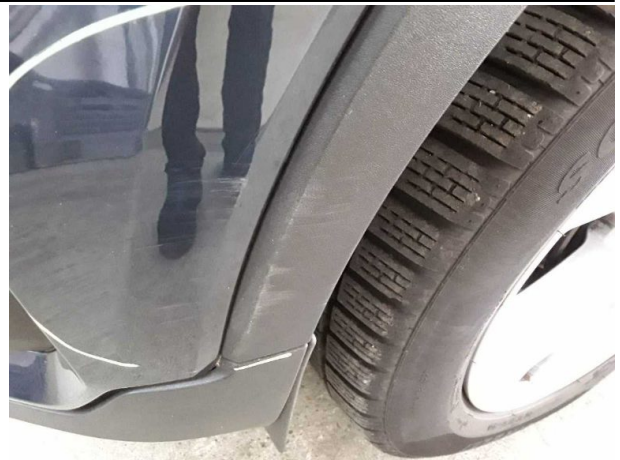
Damage #6: Mudguard - left side: Wheel well extension - Scratched - Replace
