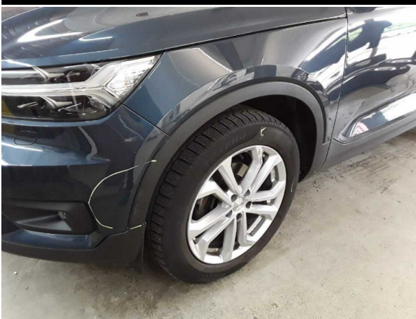
Damage #6: Mudguard - left side: Wheel well extension - Scratch... - Replace
