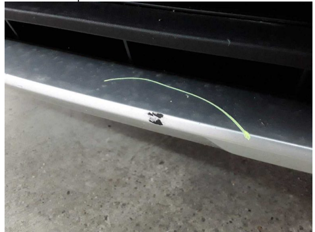
Damage #7: Front bumper: Spoiler - Scratched - Smart repair
