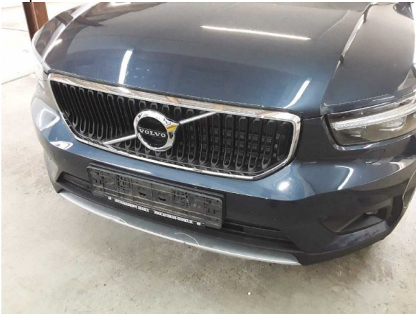
Damage #7: Front bumper: Spoiler - Scratched - Smart repair
