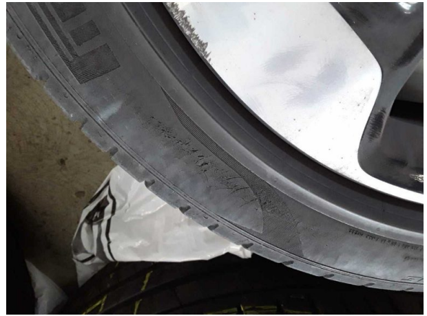
Damage #8: Wheel / tyres: Tyre - front - Damaged - Replace
