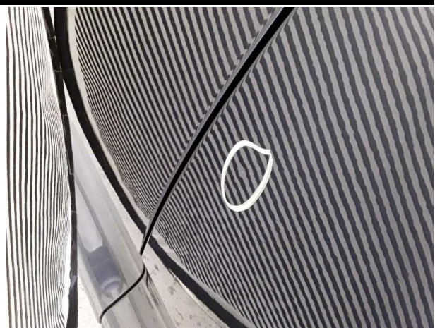
Beschädigung #4: Tür hinten links: Tür - Delle / Lackschade... Smart Repair
