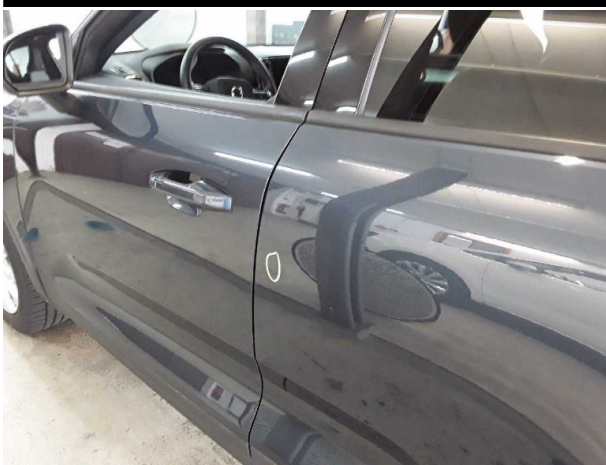
Beschädigung #4: Tür hinten links: Tür - Delle / Lackschaden - Smart Repair
