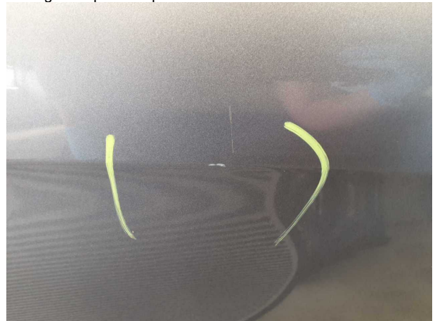
Damage #8: Door - rear right side: Door - Dent / paintcoat damage - Repair and paint
