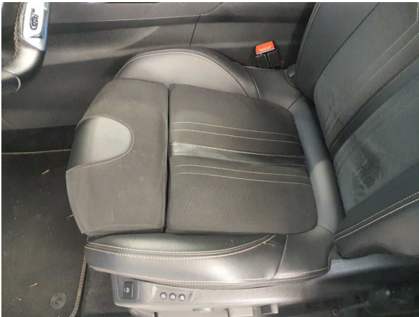
Damage #6: Seat - front: Seat cover - left side - Porous / cracked - Replace
