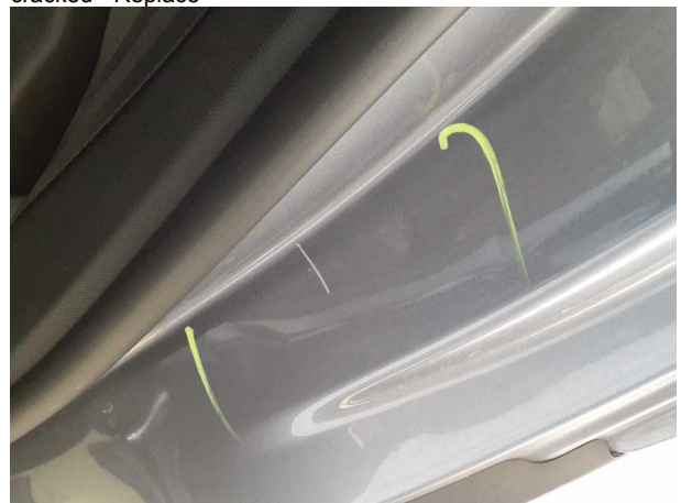
Damage #7: Side panel - rear left side: Sill - Dent / paintcoat damage - Repair and paint
