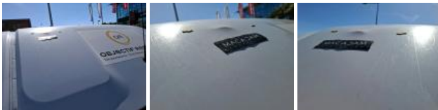
Roof, cabin, Dent(s), Repair and paint (complete)
