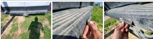
Parking sensor R, Broken, Replace
