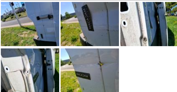
Side panel R, Dent(s), Repair and paint (complete)
